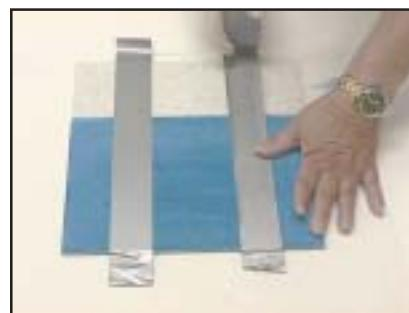
A 12" x 12" test tile is prepared by coating 2/3 of a beige/white tile with 24% finish infused with blue indicator dye. The 20 coats were applied over a 5 day period.
