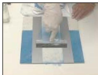
A 19-1 solution of Whax Wax and water is applied over exposed area. After 5 minutes more solution is added. No agitation.
