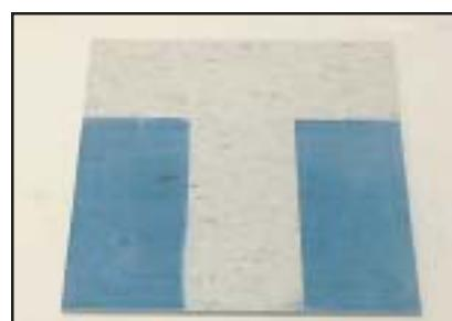
Area is wiped with a wet cloth and allowed to dry after protective tape is removed.
